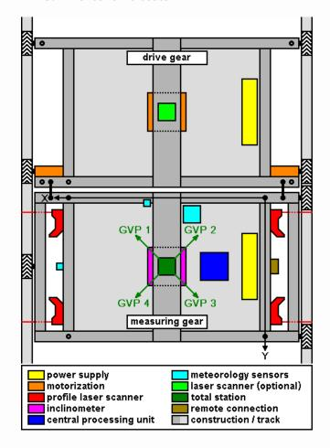
The operators monitor the complete automated process. Only the survey points along the track (called GVP) are to be equipped and aligned with precision prisms manually during the measurements.
